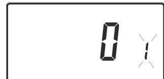
Use **Λ** and **V** keys to enable or disable the function (1=enabled, 0=disabled).
