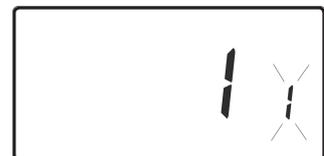
Press **PROG** for 5 seconds until the display changes and the colon in the display flashes to confirm that you are in **RUN**.
